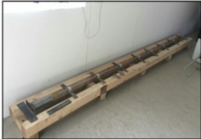
Figure :10 Split Hopkinson Bar set up (In house Development)
