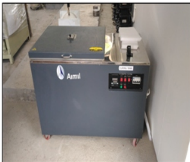
Figure :17 Curing Tank- (ii)
