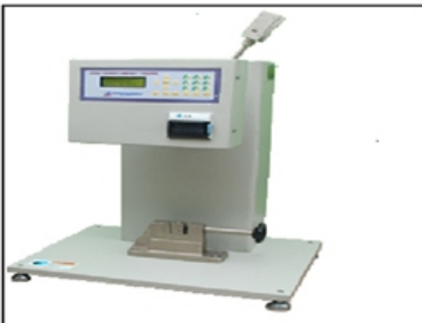
Figure :5 Izod/Charpy computerised impact tester for Polymer Composites
