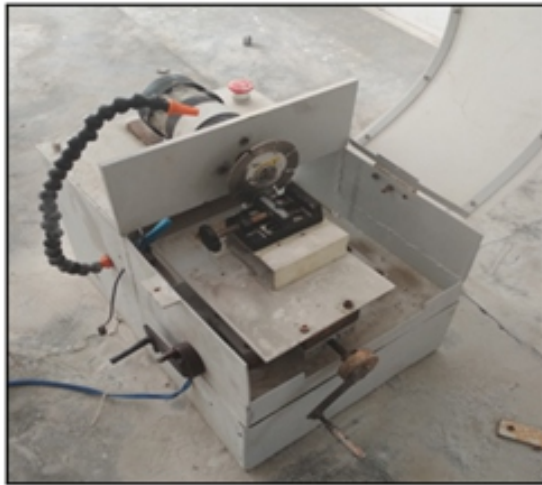
Figure :9 Precision Cutter (In house Development)
