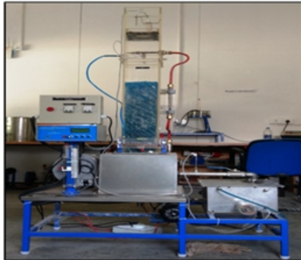
Figure :27 Water Cooling Tower
