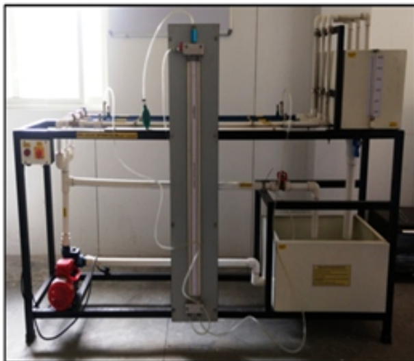
Figure :23 Pipe Losses Apparatus
