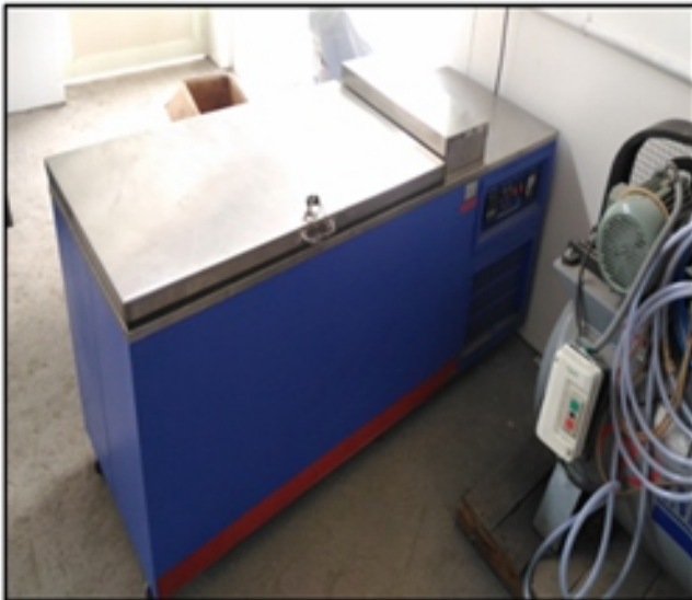
Figure :15 Curing Tank
