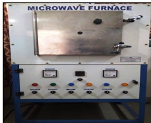
Figure :2 Polymer curing microwave applicator
